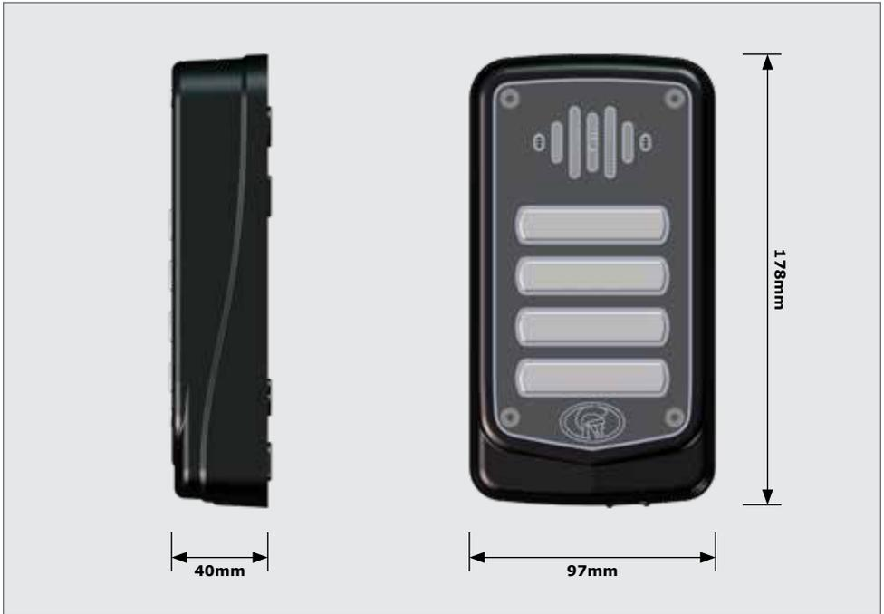
FIGURE 1. METAL GATE STATION PHYSICAL DIMENSIONS
