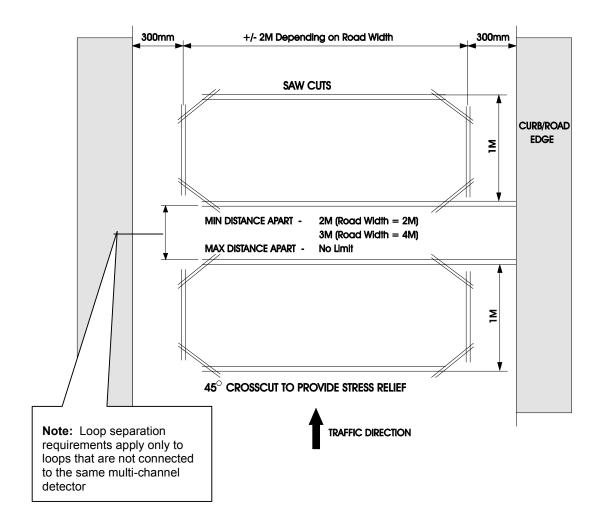
Fig 3 Loop separation requirements for loops not connected to same detector module
