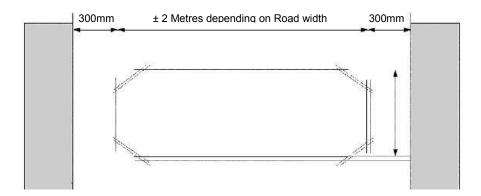
Fig 1 Loop geometry
