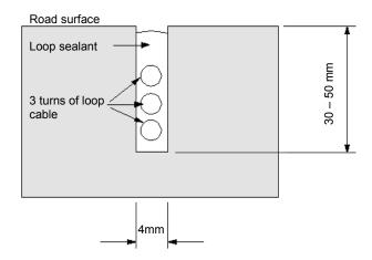
Fig 2 Loop slot detail
